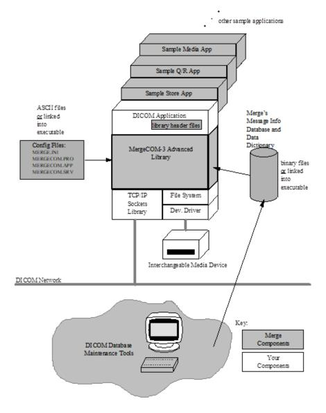
For most applications, accessing the binary files is preferred because this requires less static memory and is easier to reconfigure (does not require rebuilding executables). But, in embedded systems, where a file system is not available, statically linking in the Data Dictionary file allows attribute level (but not message level) validation, without requiring a file system.
